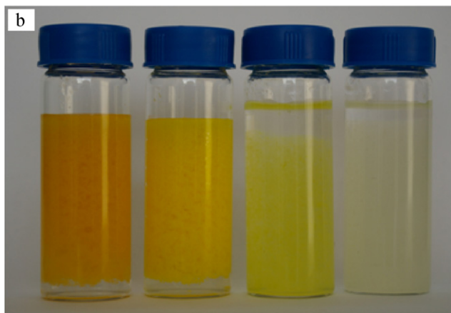
Fig. 4. (a) UV–vis absorption spectra of BC nanofibers and CdS/BCF hybrid nanofibers prepared at 180 °C for 3 h, 5 h, and 7 h. (b) Photograph image of the nanofibers and CdS/BCF hybrid nanofibers prepared at 180 °C for 3 h, 5 h, and 7 h.
